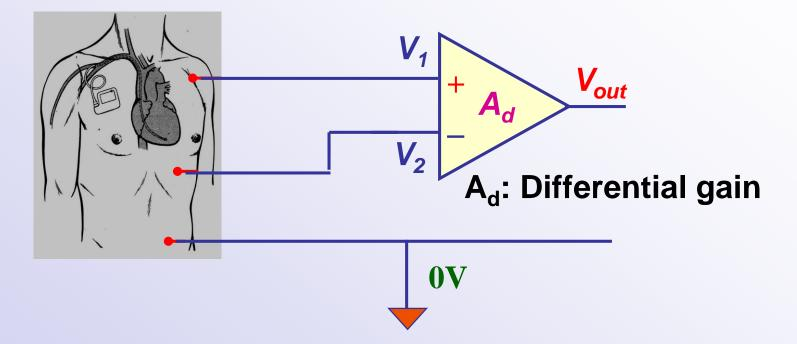
V1= CM noise + ECG V2 = CM noise Vout = Ad (V1 - V2) = Ad . ECG
